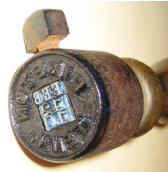
The Fiketon hand canceling device is 4.5 inches long and makes a circular date stamp one inch in diameter.
